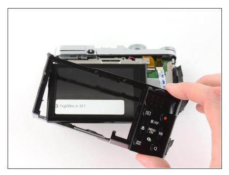
Slide the frame around the LCD to remove it from the camera.
