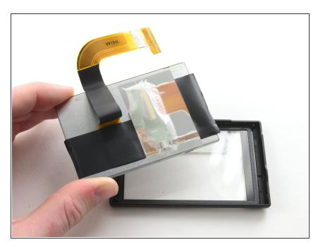
Remove the LCD from the screen cover.
