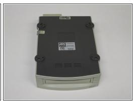
Pry all four of the plastic feet off the bottom of the enclosure using the iPod opening tool.
