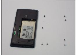
• Unscrew the 8 screws with a Torx screw driver (T4) and make sure you know what screws went where because they are different.
