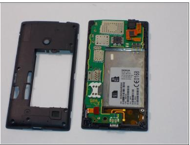
• Use your plastic spudger to remove the clips on the plastic casing over the motherboard. Note there are 10 clips holding the casing on(3 on the sides, 2 on the top and bottom).
