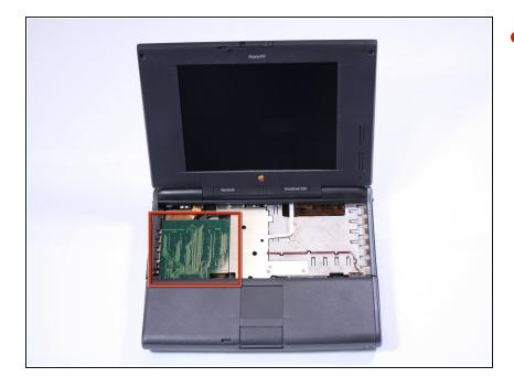
Pull up on the large green memory chip on the left side of the laptop. It will simply lift out.
