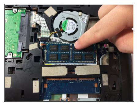
• Press down on the RAM stick and the metal clips will lock in to place.
