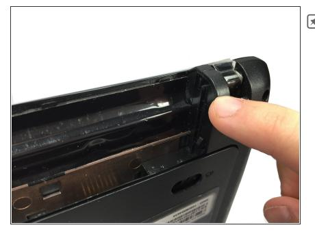
Check the thin grooves on the side of the battery entry and line the replacement battery up to the grooves.
