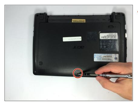
Remove the screw at the bottom of the laptop.
