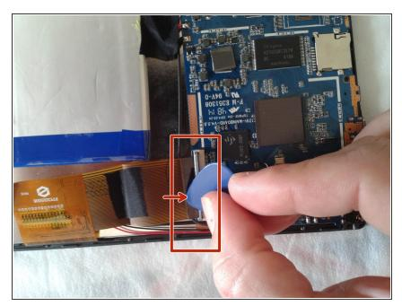
we will have a third FLEX on the motherboard, we must do the same method to press up on the connector until it is released, carefully these FLEX are easy to break.
