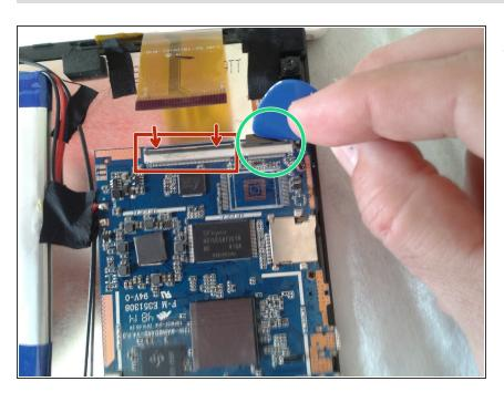
With the help of the pua or the fingers, we must release the data FLEX from the connection, making a small upward pressure
