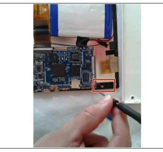
• now with the help of a Phillips screwdriver, we must release the three screws that hold the base plate of the touch screen chassis, and the sensor with positive and negative cables, we can help with the fingers in a smooth way.
