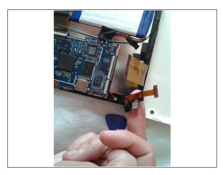
Careful! The FLEX cable that joins the front and rear camera, will be completely loose, we must place it in a clean place for later assembly.
