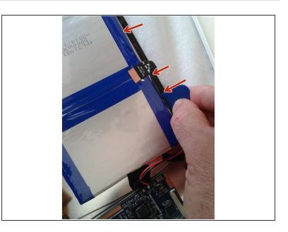
carefully, we already have the loose base plate of the touch chassis, we look at the various grips that connect the touch screen with the LCD and with the tine and small balancing we are doing pressure to separate touch and LCD screen.
