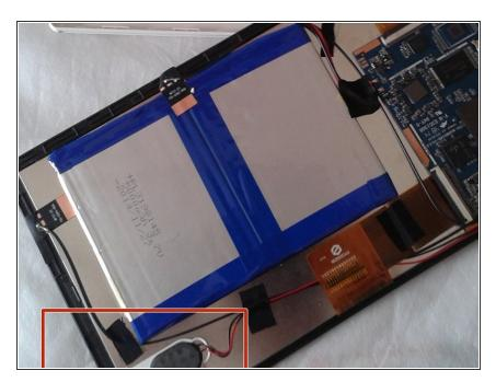
the speaker is screwed next to the touch chassis, we must release the screw and place it in a visible place, the speaker will remain with adhesive tape next to the battery
