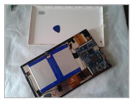
Carefully loosen with your fingers the back and place the tablet face down on a flat and clean surface tablet
