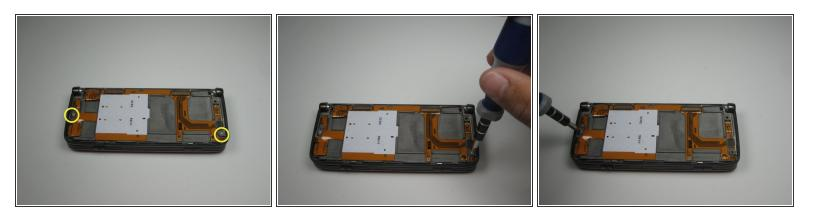
• Using the T5 Screwdriver, remove the two screws shown.
