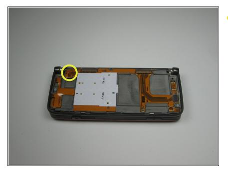
Make sure to remove the connection shown by gently easing the plastic opening tool underneath the connection and lightly prying the connection apart.
