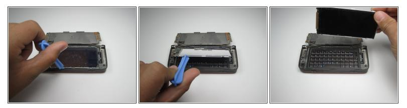
• Using the plastic opening tool, lift and remove the inside screen.
