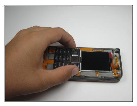
• With the front cover off, the screen and keypad should be loose.
