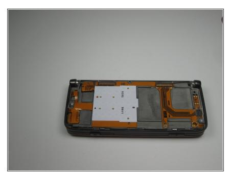
After removing the front screen and front keypad, your device should look like this.
