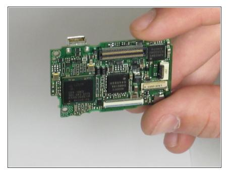
Remove the motherboard by pulling it out with either tweezers or the spudger.
