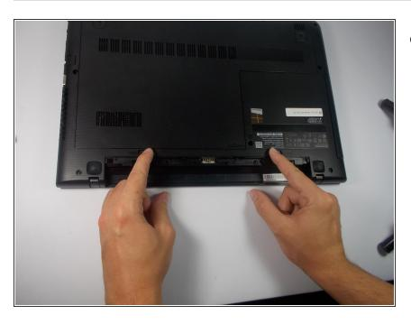
Locate the two switches above the battery.
