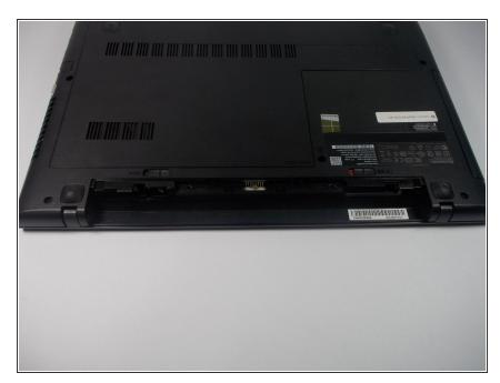
Safely place the Device upside down and have the battery component facing yourself.
