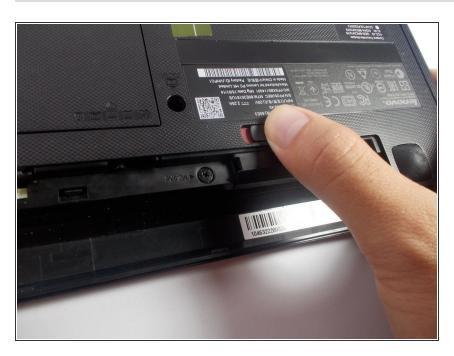
If it is not already, push the right switch to the right so that it shows a red strip. Then hold the left clip to the left and pull out the battery.
