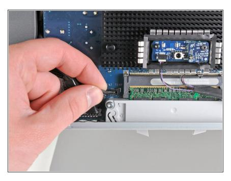
Pull the ambient temperature sensor cable out of its socket on the logic board.
