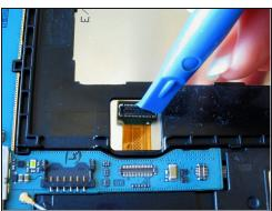
Slightly apply pressure and move the blue plastic opening tool downwards to pop the metallic rectangular connector from its socket on the mother board.
