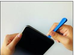
△ Before disassembling your Samsung Galaxy Tab 4 8.0, be sure it is powered off and you remove the SIM and Micro SD cards.
