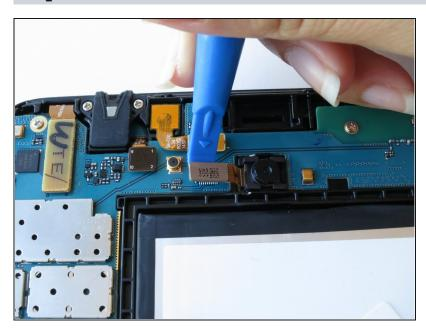
Slightly apply pressure and move the blue plastic opening tool downwards to pop the back camera's metallic rectangular connector from its socket on the logic board.
