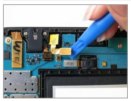
Slightly apply pressure and move the blue plastic opening tool downwards to pop the front camera's gold rectangular connector from its socket on the motherboard.
