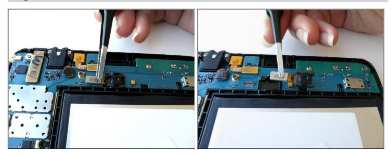
• Squeeze the metallic rectangular piece with the <u>tweezers</u> to gently lift it from it's pit.
