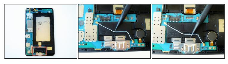
• Using the spudger gently wedge the blue wire out of its compartment.
