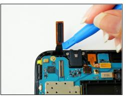
• Slightly apply pressure and move the blue plastic opening tool downwards to pop the gold rectangular connector from its socket on the mother board.
