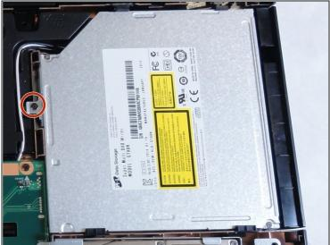
Remove the single screw that is holding the drive in place using the Phillips #1
