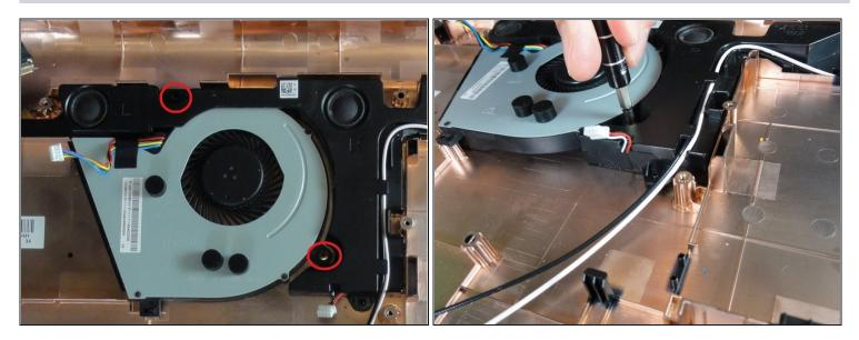
• Remove the two screws shown with the Philips #1 screwdriver.
