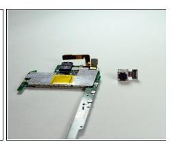
• Use the prying tweezers to remove the rear facing camera connector on its right side.
