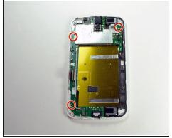
Using a T5 Torx screwdriver, unscrew the three 2.2 mm screws holding the motherboard in place.
