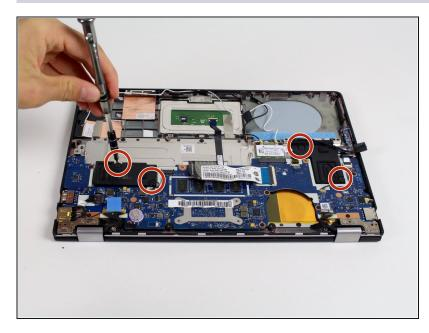
• Using a Philips 00 Screwdriver, remove the four 4.762mm screws that hold the speakers in place (two for each speaker).
