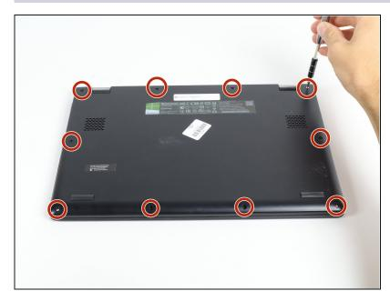
• With a T5 Torx screwdriver, remove ten 6.35 mm screws from the back of the laptop.
