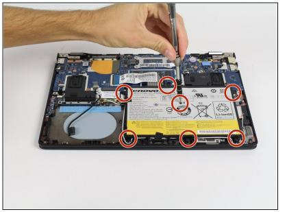
Using a #00 Philips Precision Screwdriver, remove the seven 3.175mm screws that hold the battery in place (six on the outside, one in the middle).
