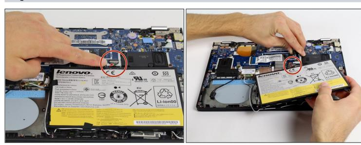
• There will be a clip that connects the battery to the rest of the laptop. Unclasp this clip by inserting tweezers into the connection to completely free the battery.
