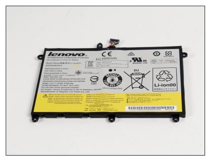
Once all of the wires are detached, carefully remove the battery and replace.
