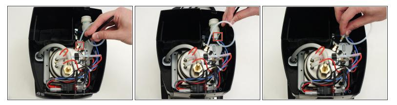
Remove each clip from the valve and core using the precision angled tweezers.
