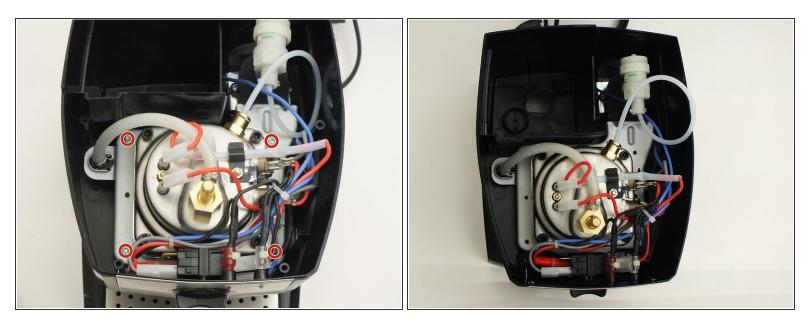
• Remove the four 16mm screws with a T20 Screw head.
