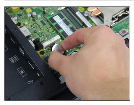
Pry the battery up from the sides to remove it.
