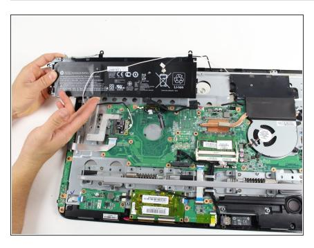
Gently remove the battery from the computer, making sure not to tug on any of the cables or wires during the removal.
