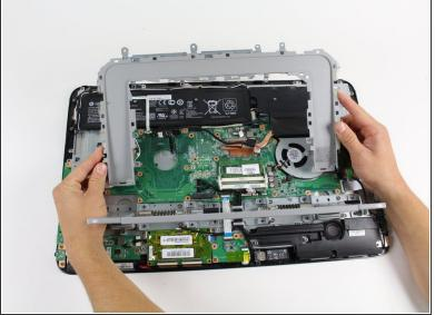
Remove the stand recess by moving it towards yourself, rotating it about the hinge and then taking it out of the computer.
