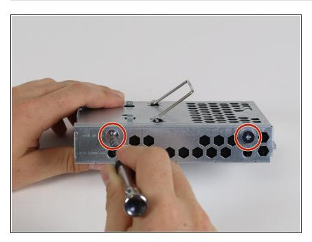
Remove the two 8.5mm PH2 screws on each side of the hard drive cover.
