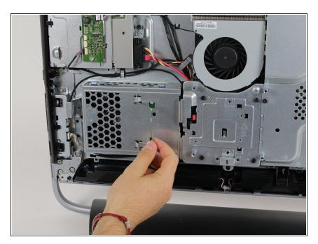
Unsnap the wire mechanism to release the hard drive.
