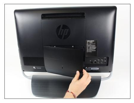
Use your hands to unclip the plastic snaps on the back panel of the device.
