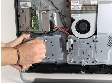
Detach the hard drive assembly by pulling it out of the socket.
