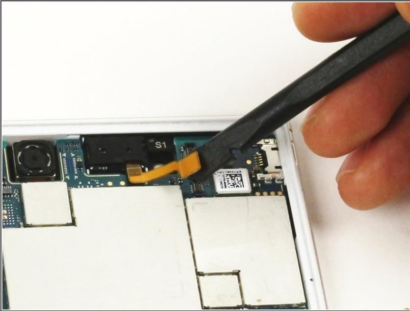
**⚠** Use care to remove the earphone jack connection, as it may snap if excessive force is used. The earphone jack connection is extremely thin.
