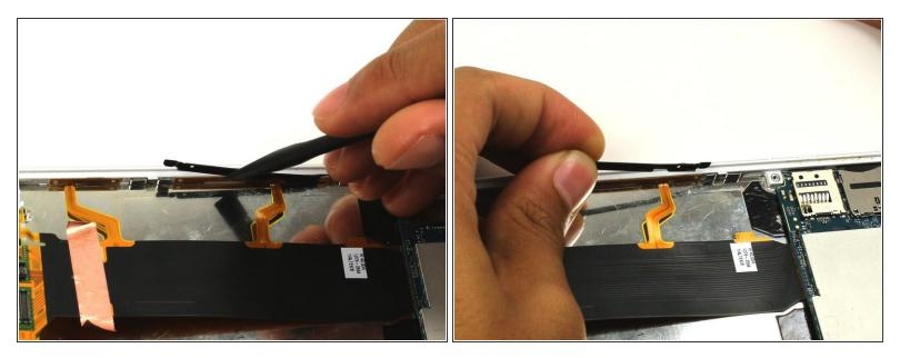
• Pry the small black metal bracket off with the spudger.
