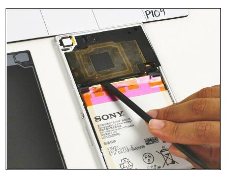
Pry the plastic motherboard shield open by placing the spudger under the shield and running it along the edges.
