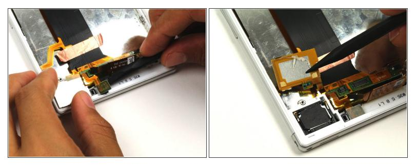
• Remove the loudspeaker connection by prying it upwards with the spudger.
