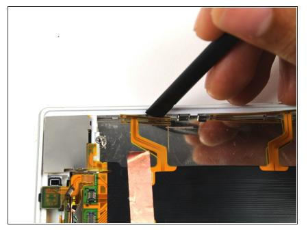
Detach smaller orange ribbon by wedging the spudger between the phone's casing and the ribbon. This will help prevent damage to the strip.
