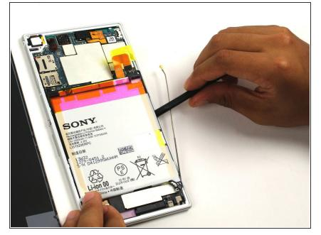
Insert the spudger underneath the battery and run it back and forth to remove any adhesive.
