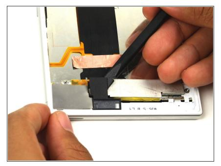
Remove the mic cover by placing the spudger underneath the cover and prying it upward.
