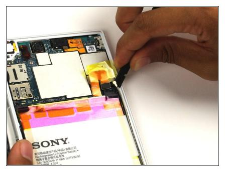
• Pry the upper end of the antenna upwards with the spudger.
