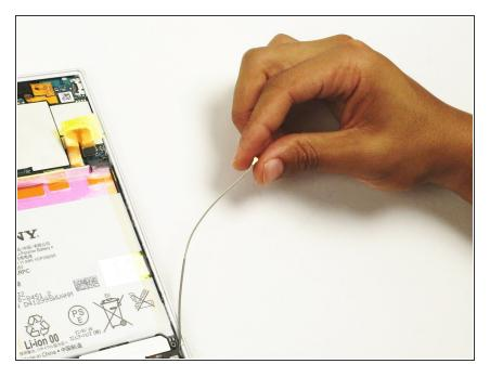
• Detach the antenna by pulling the upper end upwards and outwards.
