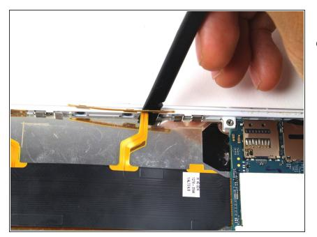
Detach the orange ribbon by wedging the spudger between the phone's casing and the ribbon. This will help prevent damage to the strip.
