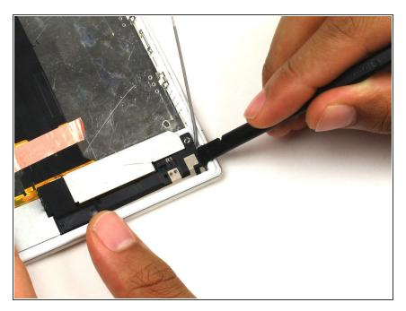
• Pry the antenna assembly upwards with the spudger.
