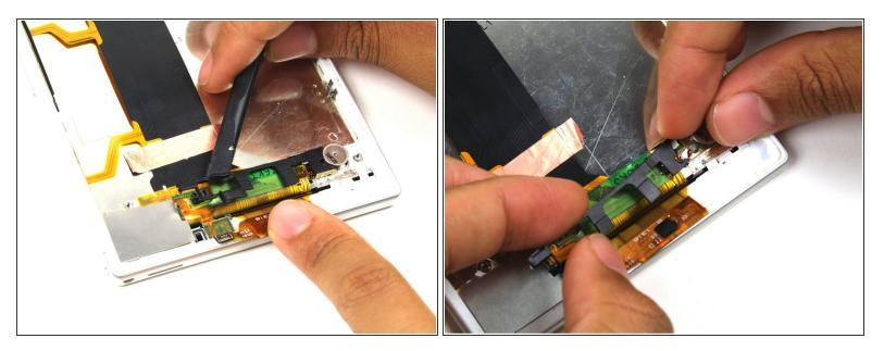
Use care to remove the black plastic spacer, as it may bend if excessive force is used. The black plastic spacer is very thin and extremely fragile.
