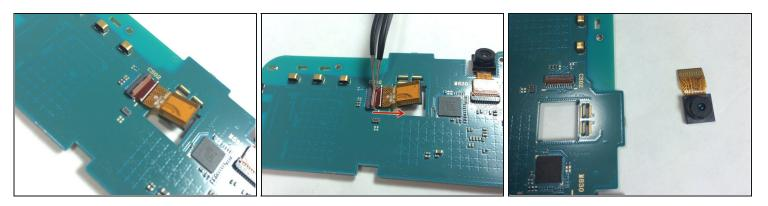
• With the <u>tweezers</u> grab the base of the wire harness and slide it outward in the direction shown.
