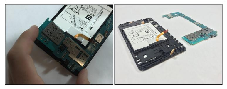
⚠ Use extreme care while removing the motherboard to avoid damaging the component.
