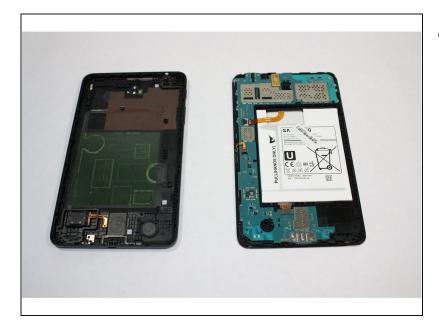
• Carefully separate the rear housing from the front panel assembly.
