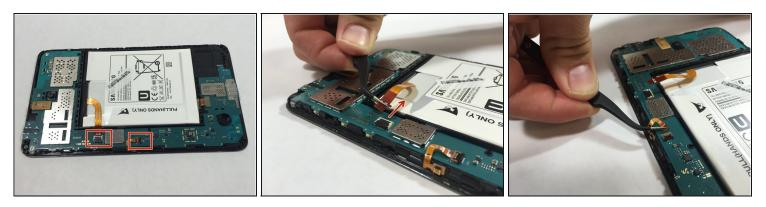
• Using the bent <u>tweezers</u>, carefully pull the flat cables away from the connectors.
