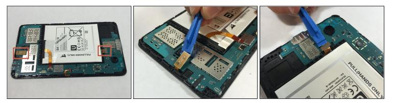
• Using the plastic opening tool, gently pry the chip connections away from the motherboard.
