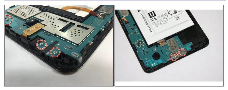
• Use the Phillips 000 screwdriver to remove the remaining five 1.2 mm screws.
