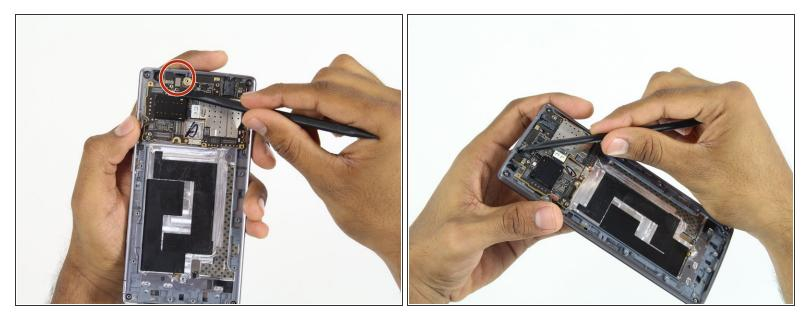
• Use the spudger tool to pry up the connection at the top of the motherboard.
