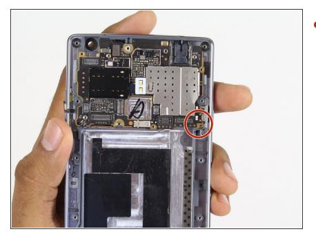
Use the screwdriver to unscrew the screw fastened at the bottom right of the motherboard.
