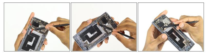
• Use the spudger tool to pry off the 2 connections at the bottom-left of the motherboard.
