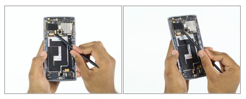
• Use the spudger tool to pry off the connection on the left of the front facing camera.
