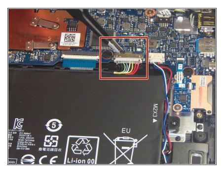
Use a pair of tweezers to gently disconnect the battery connector.
