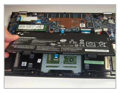
Carefully remove the battery from the device.
