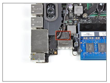
Remove the small piece of black tape covering the left speaker connector.
