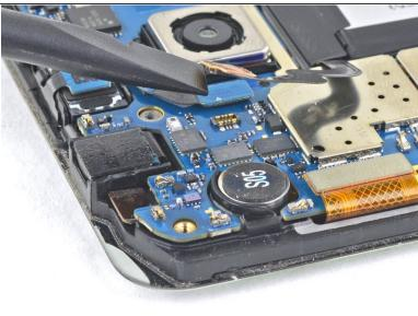
Using the flat end of a spudger, lift the battery connector straight up from its socket on the motherboard.
