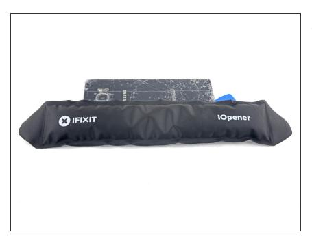
Before cutting further, apply a heated iOpener to the long edge.
