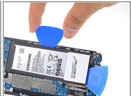
Slide an opening pick up the side of the battery to break apart any remaining adhesive.
