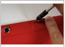
Remove the 5 mm screw using the Phillips PH00 bit in the iFixit metal Screwdriver.
