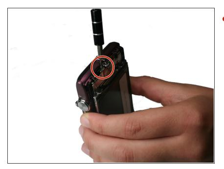
Using the Philips #000 head screwdriver, remove the 1.90 mm internal screw located just above the lanyard mount.
