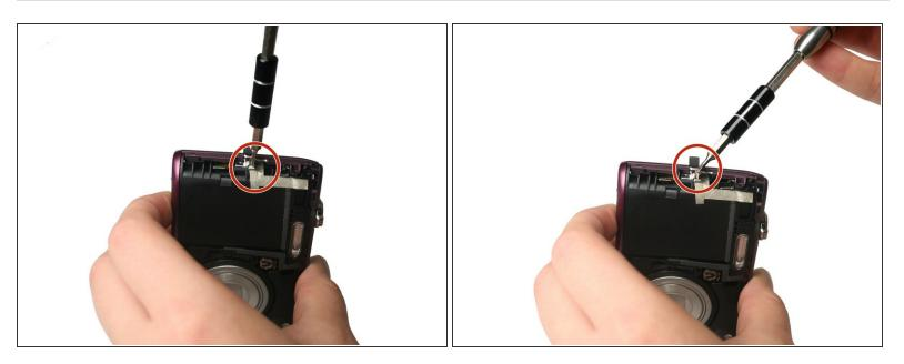
Using the Philips #000 head screwdriver, remove 2 additional 3.30 mm screws holding the lanyard mount in place.
