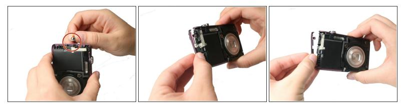
• Remove the lanyard mount and accompanying side shell casing off of the camera.
