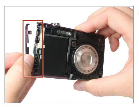
Remove the remaining side shell casing.
