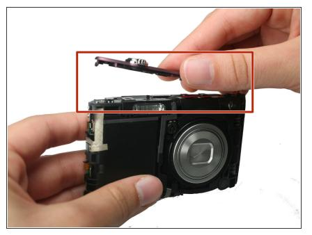
• Remove the top shell casing.
