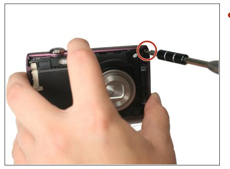
Using the Philips #000 head screwdriver, remove the 3.40 mm screw located on the front of the camera in the upper corner by the LED light.
