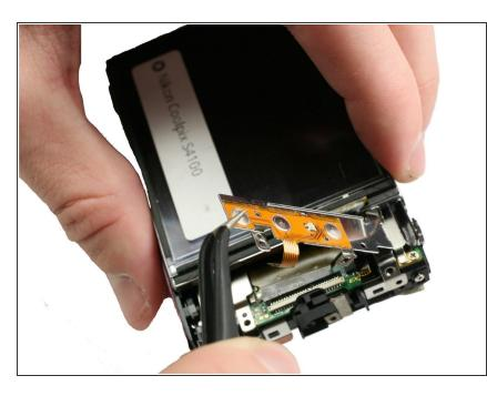
• Using precision tweezers, lift up the bottom of the functional buttons plate and remove the metal plate.
