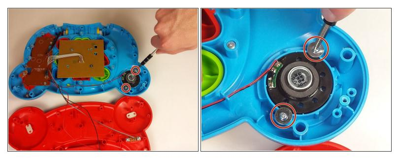
Use a Phillips #0 screwdriver to unscrew the two 6.0 mm screws on the speaker.
