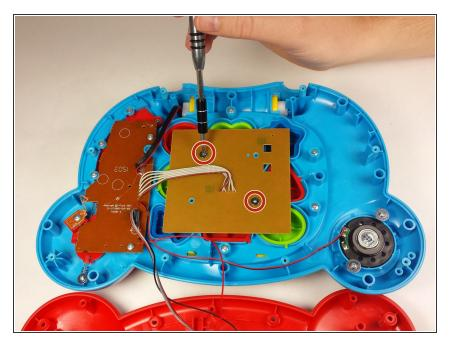
• Using a Phillips #0 screwdriver remove the two 6.0mm screws.
