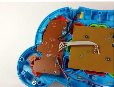
Using a Phillips #0 screwdriver, remove the three 7.3mm screws.
