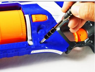
Locate the 12 Philips head screws and remove them: Head Diameter= 4.3mm, Thread Pitch= 1mm, Screw Length= 8mm
