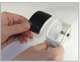
Remove the wrist strap by peeling back the rubber starting from one corner of the watch face.
