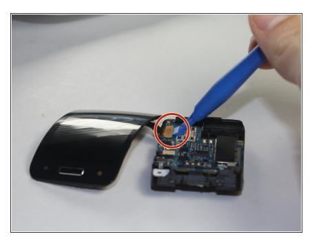
Use a plastic opening tool to detach the glass screen/ LED Display ribbon connector from the motherboard.
