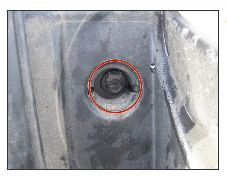
Once covers are removed, there will be an 8 mm hex head screw located beneath each cover.
