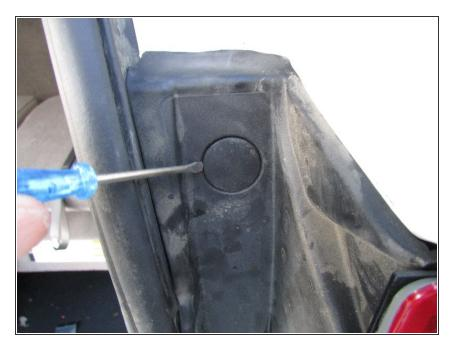
Using a flathead screwdriver, pry out both plastic screw covers.
