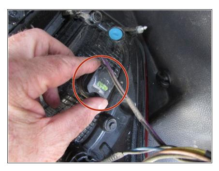
Once removed, the bulb sockets will be located on the inside portion of the tail light cover.
