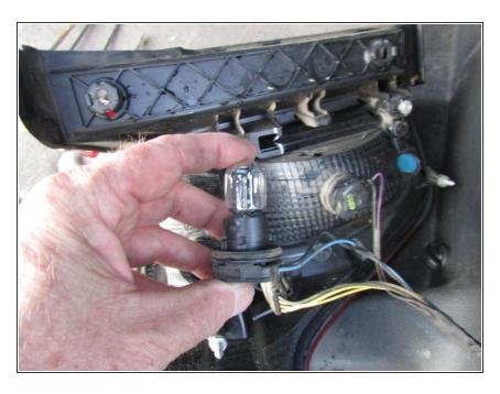
Gently place the new bulb in the bulb socket.
