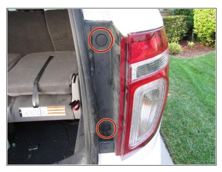
Locate the two plastic screw covers that are adjacent to the rear light covers.
