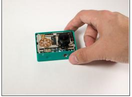
Slide prying tool along the seam until front panel is fully separated from the back panel.
