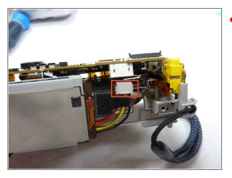
• Remove the cable on the back side of the motherboard.
