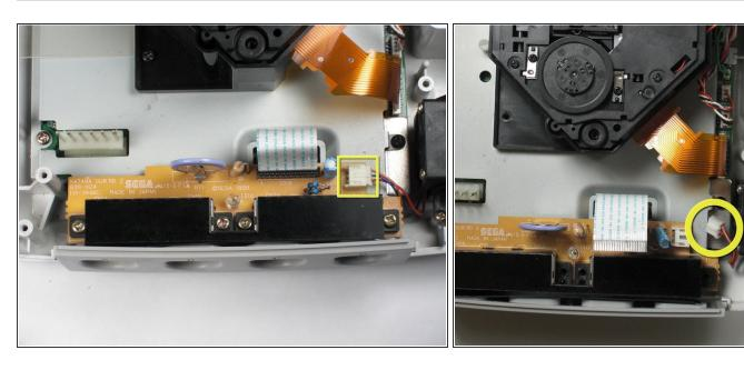
Disconnect the white fan header from the controller port.
