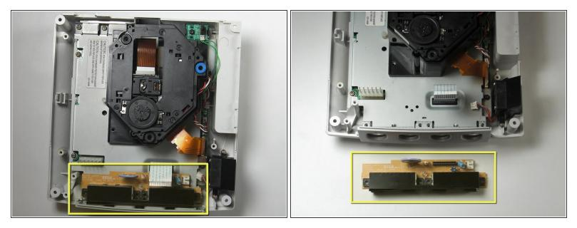
Remove the controller board by lifting it up from the controller port.
