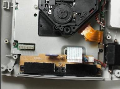
Remove the four 14mm Philips #02 screws located on the controller board.
