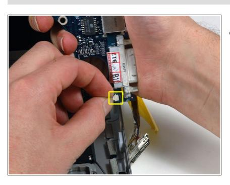
Disconnect the right thermal sensor cable from the bottom of the logic board near the DVI port.
