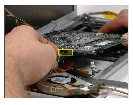
Lift up the left side of the logic board and disconnect the multi-colored power cable from the bottom of the board.
