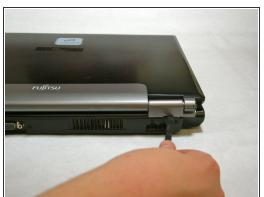
• Use a spudger to lift the back of the hinge cover on the left and right sides of the computer.
