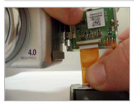
Unplug the ribbon cable connected to the circuit board latch.
