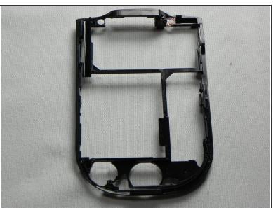
• Finally the mother board can be removed from the center black frame.
