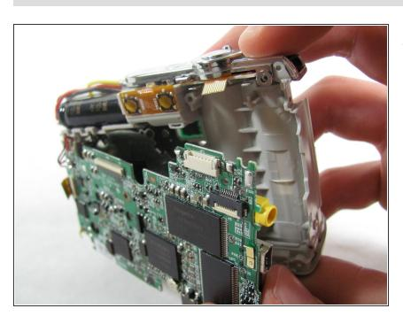
Remove the motherboard from the camera casing.
