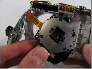
• Slide the lens to the left and pull up. The lens should easily come loose and slide right out.
