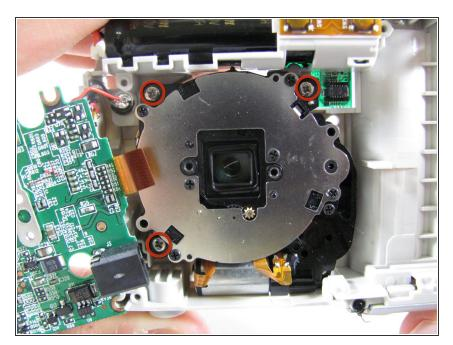
Remove the three 3.6 mm screws using a #00 screwdriver.
