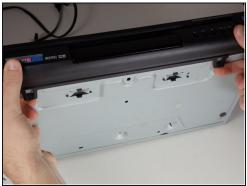
• There are six symmetrically placed tabs holding in the front faceplate. Unhook these six tabs to loosen the faceplate.
