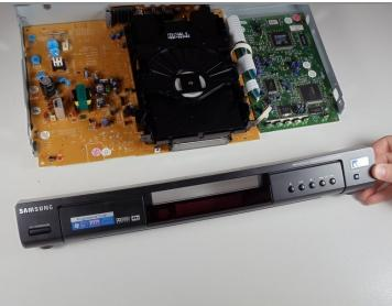
• Pull off front faceplate. This may take a couple of tries to get all six tabs unhooked simultaneously.
