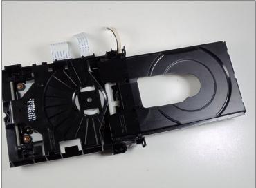
• Spin the small gear shown to the right to begin opening the tray. There should be relatively little resistance in the gear.
