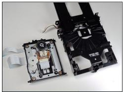
• Use your fingers to pull the shown tabs towards the sides of the tray, releasing the internal tray that contains the laser.
