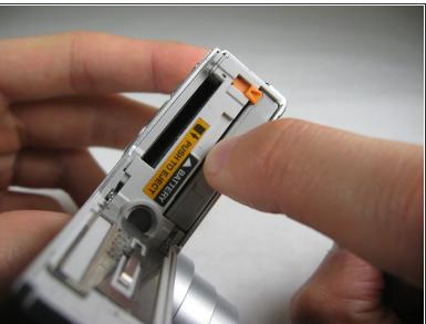
To reinsert battery, if necessary repeat Step 1. Insert battery so that the side of the battery with "CAUTION" below the black bar with an arrow faces the label "BATTERY". Make sure to push battery until small, orange lever holds battery in place. Close battery cover.
