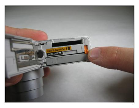
Push small, orange lever up to release battery.
