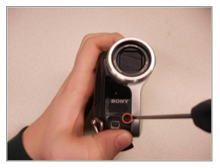
Remove the 4.5 mm screw under the output flap on the front of the camera below the lens.
