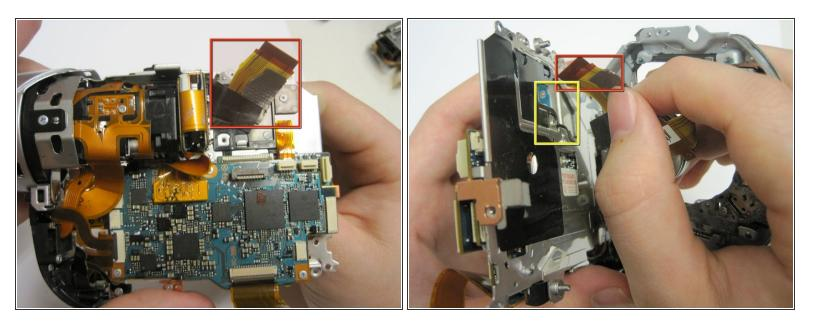
Pull the copper strip, marked by the red rectangle, through the hole behind it, marked with the yellow rectangle.
