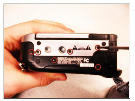
Using a #00 Phillips screwdriver, remove the six 4.5 mm screws from the camera's bottom.
