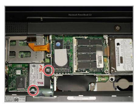
Remove the two silver Phillips screws from the modem.
