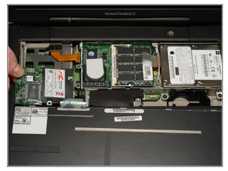
Use a spudger, the tips of your fingers, or a flat non-metal tool to get under the modem's edge and pry it up from its socket as shown in the picture.
