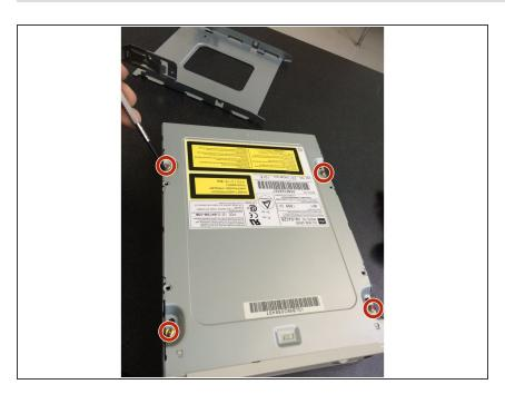
Unscrew the four screws on the next plate.
