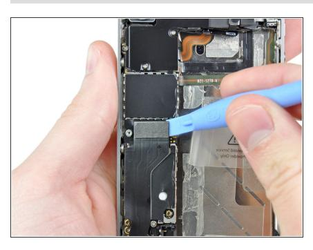
Use the edge of a plastic opening tool to pry the dock cable up from its socket on the logic board.
