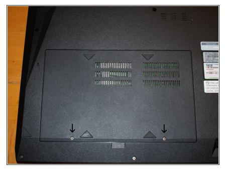
Remove the two screws indicated to remove the access panel. I recommend keeping the screws with the panel so you don't lose or forget them.
