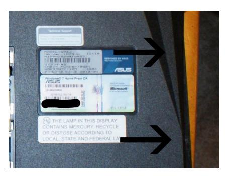
With the optical drive removed, there are two screws now accessible, indicated by the black arrows.
