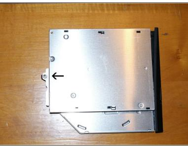
• Indicated by the white arrow is the screw to remove to allow you to pull the optical drive. Also visible beneath the screw hole is a silver tab. Push this to the right to get a grip on the drive door and pull it the rest of the way out. When the drive is removes, put the screw back in the hole in the drive, to keep track of it.
