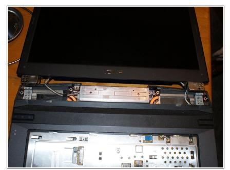
• When the screws are removed, gently pull the LCD panel up, then rotate it back so that it lays flat. Take care not to place undue stress of the cables still connecting it to the rest of the laptop.
