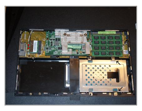
With the panel removed, we get our first glimpse to the inner workings. Note the bay for the second hard drive in the lower left-hand corner, and the existing system drive in the lower right-hand corner. The black arrows indicate the two screws to remove, allowing you to pull the drive out of the unit by grasping the black plastic tab and gently pulling to the left. Remove the WLAN card in the upper left-hand corner by removing the two screws indicated
