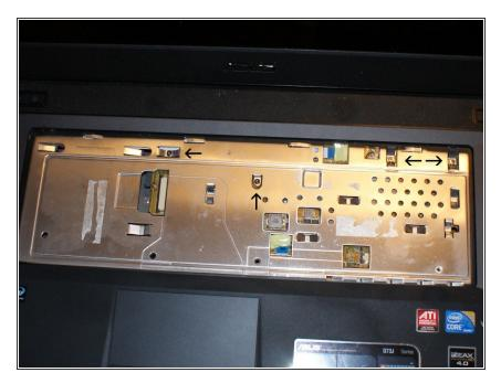
Here is the top cover, sans keyboard. Remove the four screws holding it in place.
