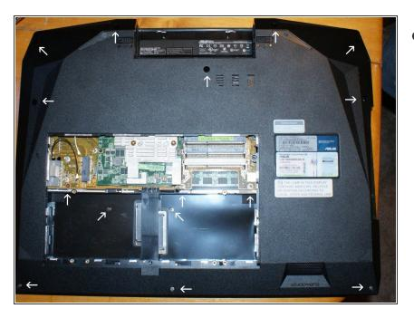
The white arrows indicate the screws to remove. There should be 15 screws.
