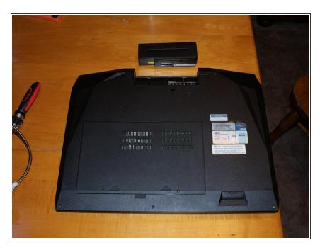
Here's where we start. Flip the notebook over onto its back with the front edge towards you. Remove the battery, we won't be needing it for a while...
