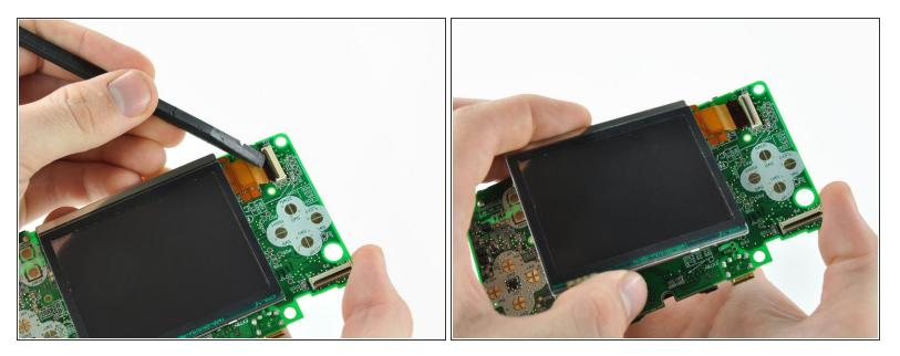
• Use your fingernail or the edge of a plastic opening tool to carefully flip up the lower LCD ribbon cable retaining flap.
